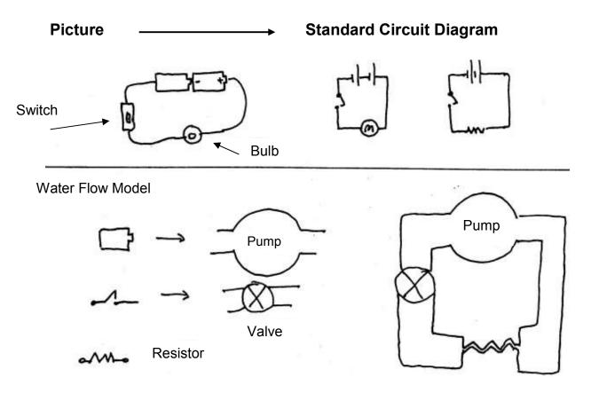
A battery is like a pump. It does not make electrical charge, just as a pump does not make water, but both push the quantities through their circuits.
